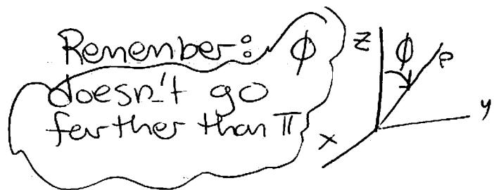
$$\begin{aligned}x &= \rho \sin \theta \cos \phi \\y &= \rho \sin \theta \sin \phi \\z &= \rho \cos \theta \\x^2 + y^2 + z^2 &= \rho^2 \\dV &= \rho^2 \sin \theta d\rho d\theta d\phi\end{aligned}$$
