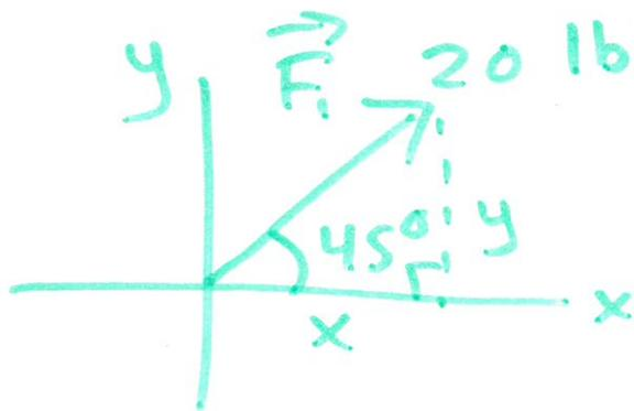
★ Basically we need to break  $\vec{F}_1$  up into its horizontal & vertical components
